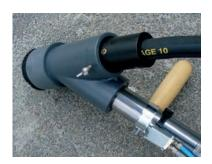
Recycling is possible depending on the support and the kind of media. Boron carbide nozzles are recommended for corundum.
