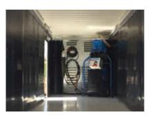
Recycling: 1 pneumatic vacuum cleaner adaptable on the technical unit and hopper extension positioned above the sandblaster
